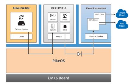
Three solutions combining an IEC 61499-compliant PLC with cloud connectivity for common Security concerns in edge devices.
